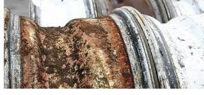
**Never** reinflate any tire that has been operated in a runflat or underinflated condition (i.e. 80% or less of recommended operating pressure).
