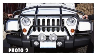
2. Carefully lower the Over-The-Hood Bar Section onto the Grille Guard Receiver Posts. Continue to support the Over-The-Hood Bar Section. (See Photo 2)
