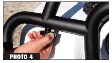
**4.** Thread Quick-Release Bolt with washer from underside of Grille Guard and into Over-The-Hood Bar Section. Tighten securely. Note: Do not overtighten. (See Photo 4) Repeat for other side.
