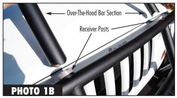
1. Carefully position the Over-The-Hood Bar Section onto the top of the Grille Guard, aligning middle vertical bars over the Receiver Posts on the Grille Guard. (See Photos 1A & 1B)
