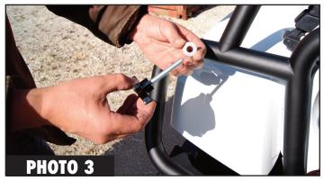
**3.** Once the Over-The-Hood Bar Section is in the Receiver Posts, slip washer onto Quick-Release Bolts. (See Photo 3)
